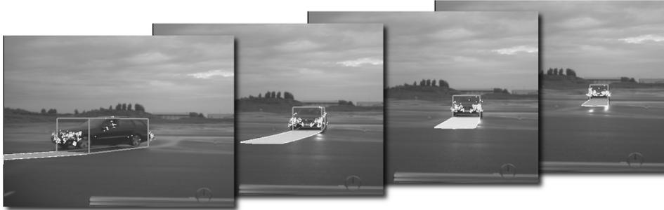
**Fig. 2:** Estimation results of an oncoming vehicle first detected at 48 m distance. The predicted driving path indicating curve radius and velocity for the next second and the tracked 3D points are shown as well as a bounding box indicating the object pose.
